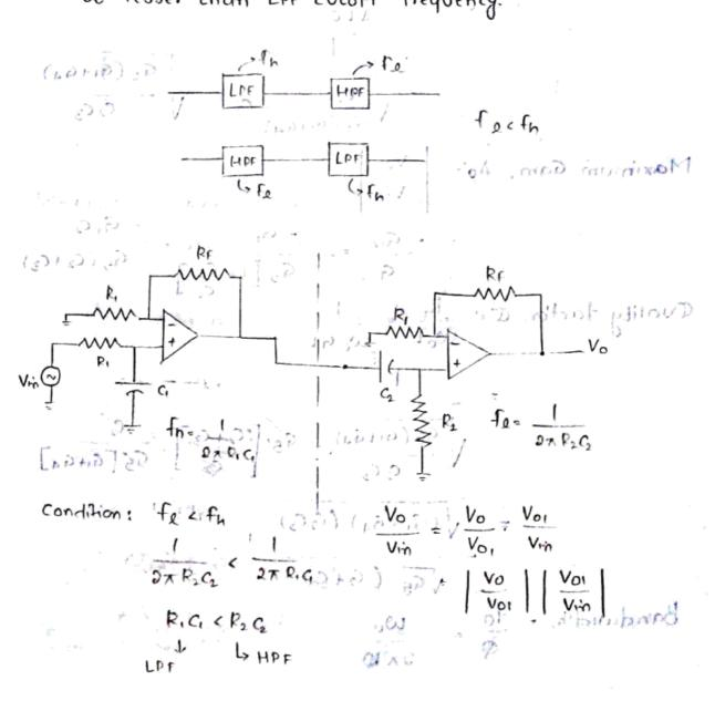
$$\frac{V_0}{V_{in}} = \frac{V_0}{V_{01}} \cdot \frac{V_{01}}{V_{im}}$$
